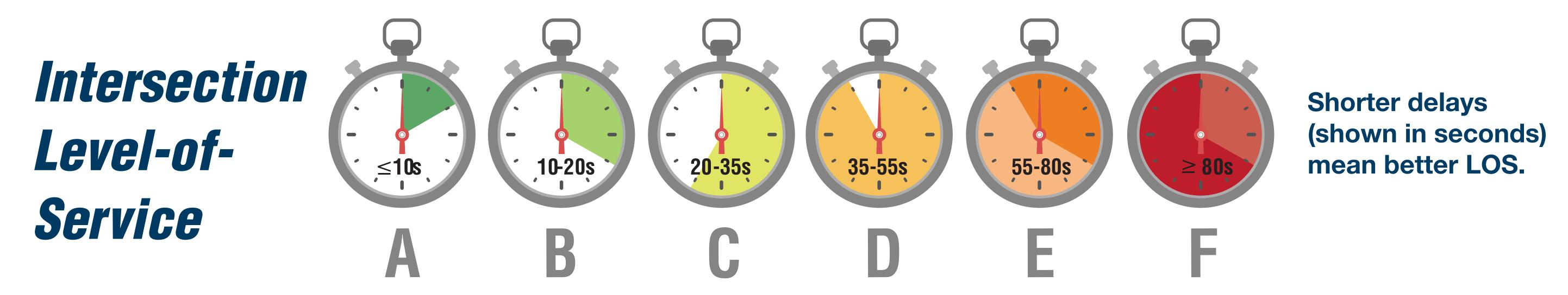
LOS F describes very congested driving conditions where the number of vehicles arriving at an intersection exceeds the capacity of the intersection. Most drivers have to wait for multiple green lights before they get through the intersection. Long queues of left turning vehicles stack out of the left turn pockets and block adjacent through lanes.
